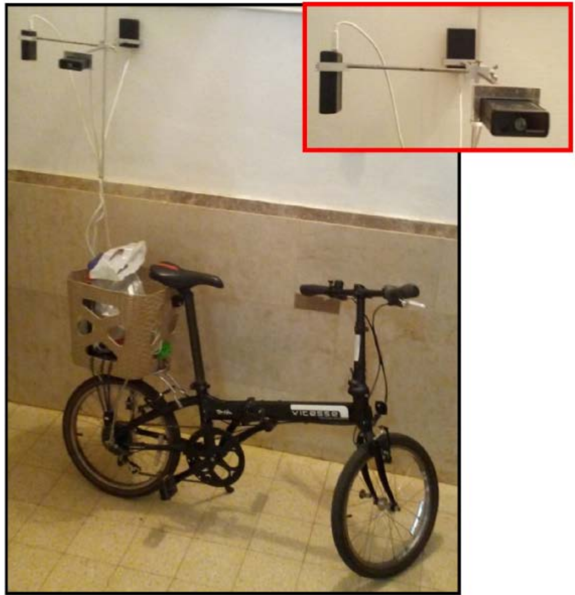
Fig. 2. Setting of the three SQM devices for ground measurements of light pollution, pointing in three viewing directions on a specially designed pole which was mounted on a bicycle.
