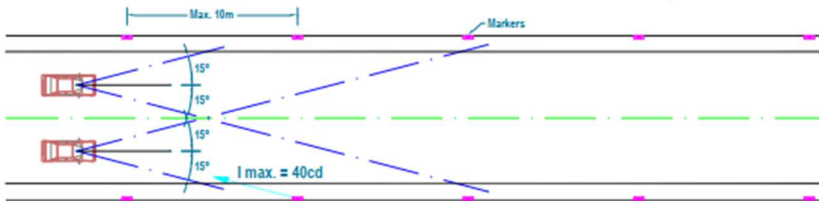
Figure 5. Limitation of intensities emitted towards driver. (Plan view showing cone of limited intensities and markers)
